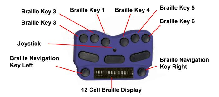
The navigation key located on the left and right of the Braille line are for scrolling the Braille display. Pressing the left and right Braille navigation keys simultaneously will move the cursor to the beginning of the Braille display. The joystick allows you to arrow up, down, left or right. Pressing the joystick will perform an Enter.
