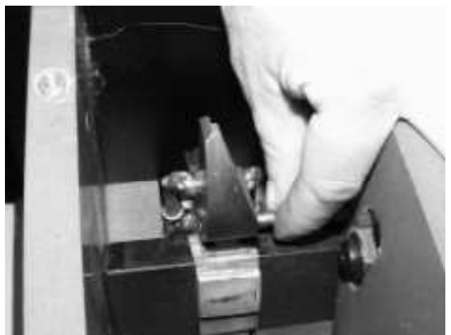
Fig. 52-3 Remove axis pin
