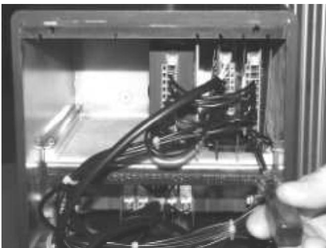
Fig. 55-6 Plug in all control plugs and tighten it by the screws.
