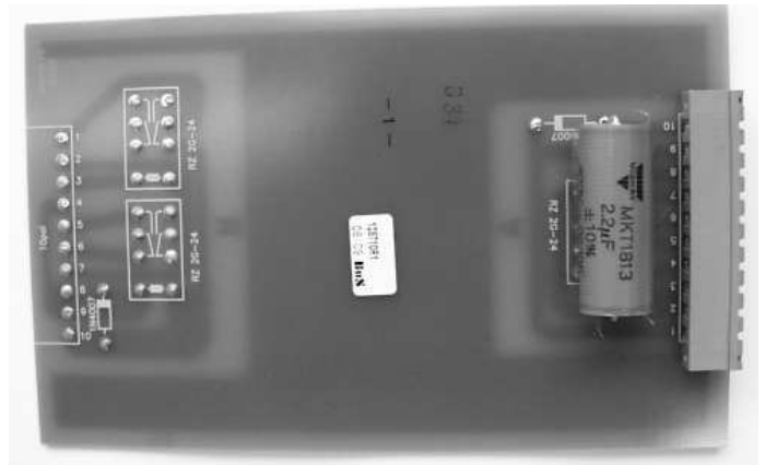
Fig. 19-4c Extinguish capacitor for direct ST supply.
