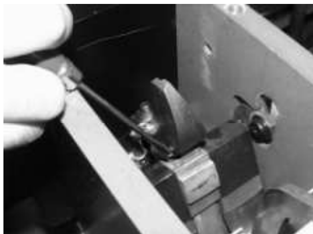
Fig. 52-1 Unscrew cooper braid
