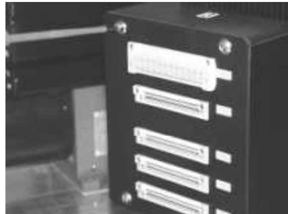
Fig. 55-2 Unscrew four bolts of the box cover
