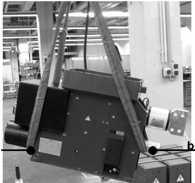
Fig. 1 Handling the breaker
