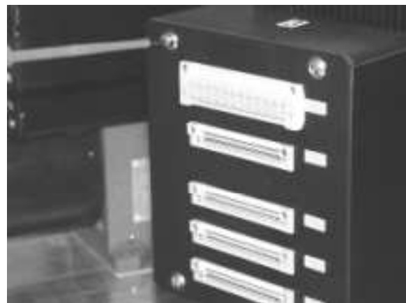
Fig. 55-8 Carefully replace the control box front cover and attach the with the four screws
