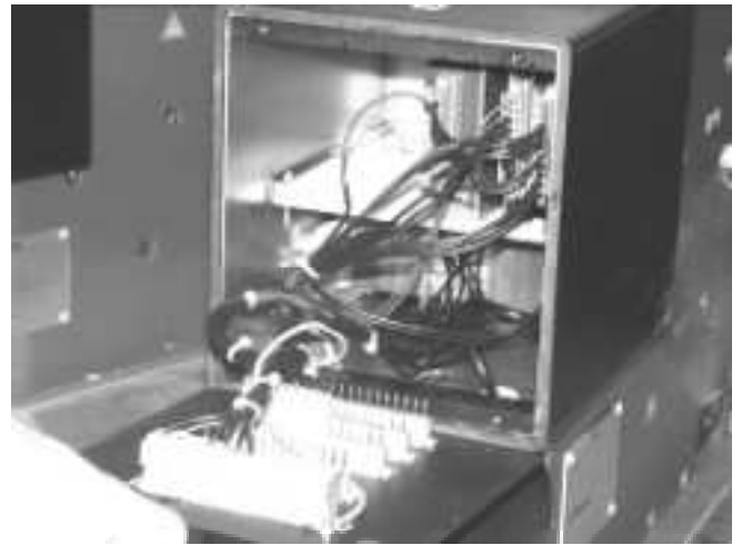
Fig. 55-7 Pay attention, that no cables will be pinched between box and front cover during closing!
