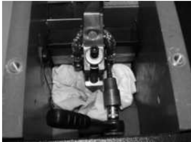
Fig. 52-1 Unscrew cooper braid
