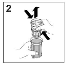
After cleaning the filters, make sure that they are correctly reassembled and that the gauze filter is properly positioned at the bottom of the dishwasher.
