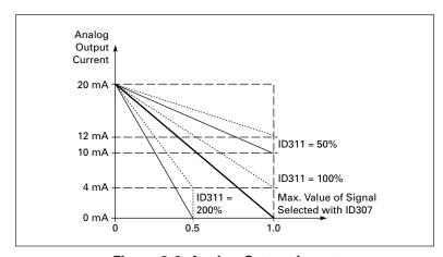
Figure 9-6: Analog Output Invert
