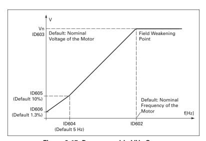
Figure 9-17: Programmable VHz Curve
