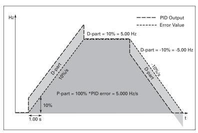
Figure 9-27: PID Output with the Values of Example 3
