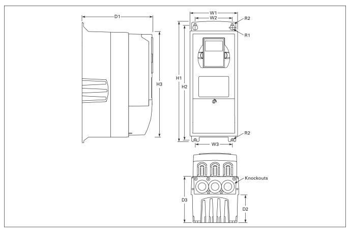
Figure 2-1: NEMA Type 1 and NEMA Type 12 SLX9000 Drive Dimensions, MF4 – MF6
