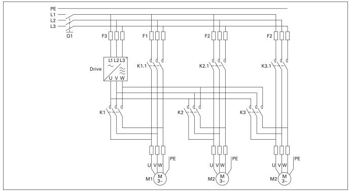
Figure 9-31: Example of 3-Pump Autochange, Main Diagram
