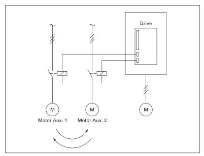
Figure 9-34: Autochange Applied to Auxiliary Drives Only
