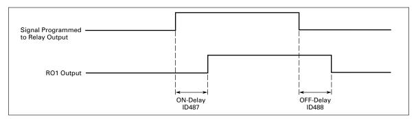
Figure 9-9: Relay Output 1 ON- and OFF-Delays
