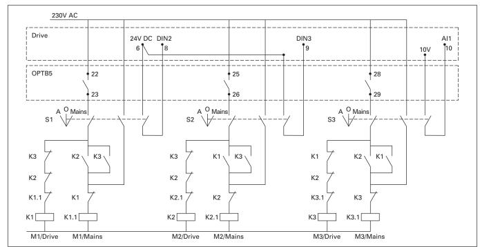
Figure 9-30: 3-Pump Autochange System, Principal Control Diagram
