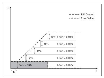
Figure 9-25: PID Controller Function as I-Controller
