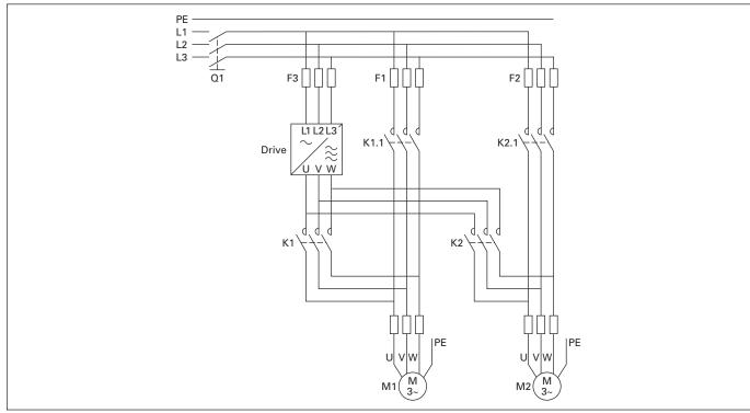
Figure 9-33: Example of 2-Pump Autochange, Main Diagram
