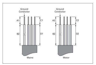
Figure 3-5: Stripping of Cables
