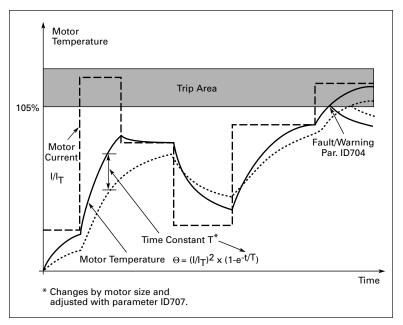
**Figure 9-19: Motor Temperature Calculation**
