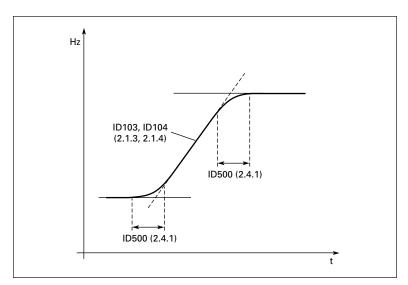
Figure 9-10: Acceleration/Deceleration (S-Shaped)
