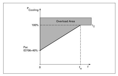
Figure 9-18: Motor Cooling Power
