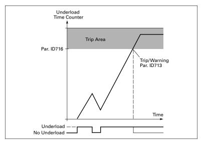
Figure 9-23: Underload Time Counter Function
