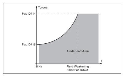
Figure 9-22: Setting of Minimum Load
