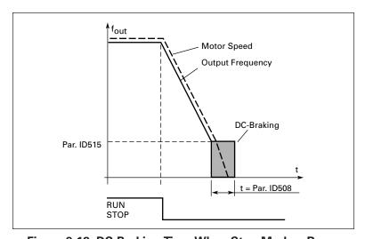
Figure 9-12: DC-Braking Time When Stop Mode = Ramp
