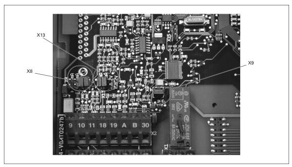
Figure 4-5: Location of Jumper Blocks in the Control Board of MF4 - MF6, 460V
