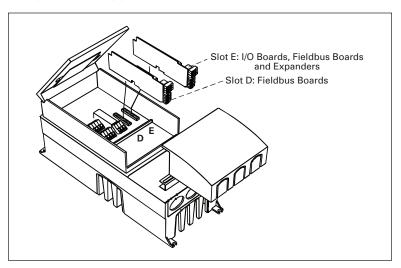
Figure 4-1: Option Board Slots D and E in Frames MF4 – MF6 460V only.
