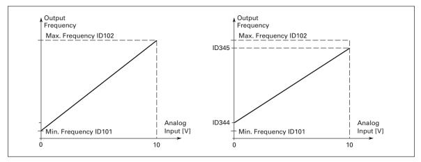
Figure 9-4: Without (Left) and With (Right) Reference Scaling
