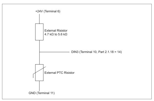
Figure 4-6: Motor Thermistor (PTC) Connection
