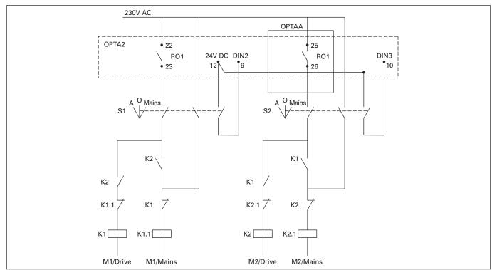
Figure 9-32: 2-Pump Autochange System, Principal Control Diagram
