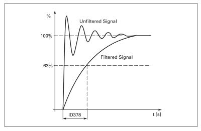
Figure 9-3: Al1 Signal Filtering
