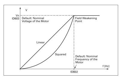
Figure 9-16: Linear and Squared Change of Motor Voltage
