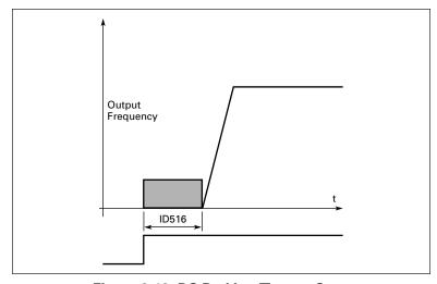
Figure 9-13: DC Braking Time at Start
