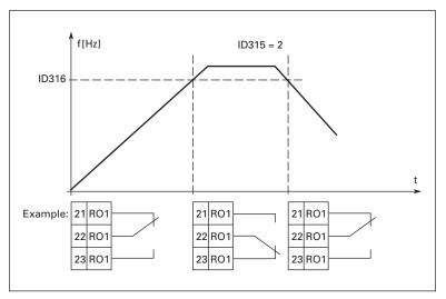
Figure 9-8: Output Frequency Supervision
