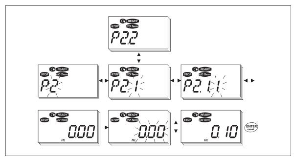
Figure 5-6: Parameter Value Change Procedure
