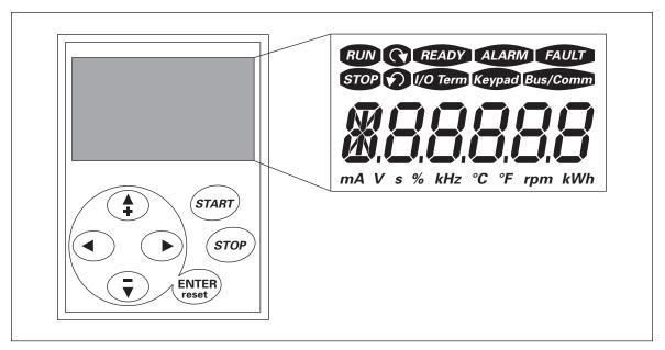
Figure 5-1: Control Keypad and Drive Status Indications
