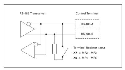
Figure 5-18: Modbus Interface
