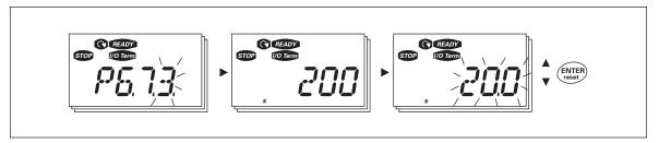
Figure 5-15: HMI Acknowledge Timeout
