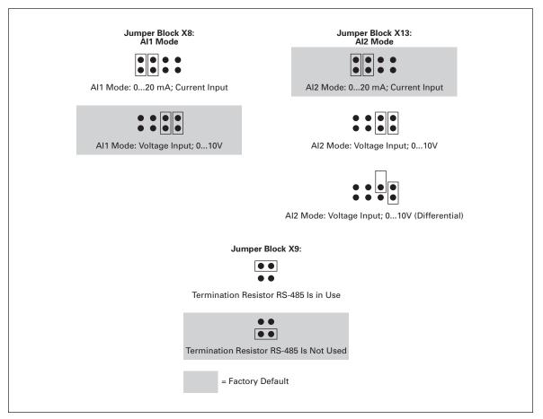
Figure 4-4: Jumper Selection for SLX9000, MF4 - MF6
