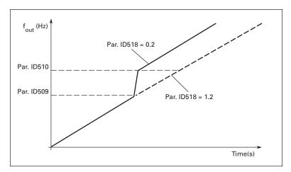
Figure 9-15: Ramp Speed Scaling Between Prohibit Frequencies
