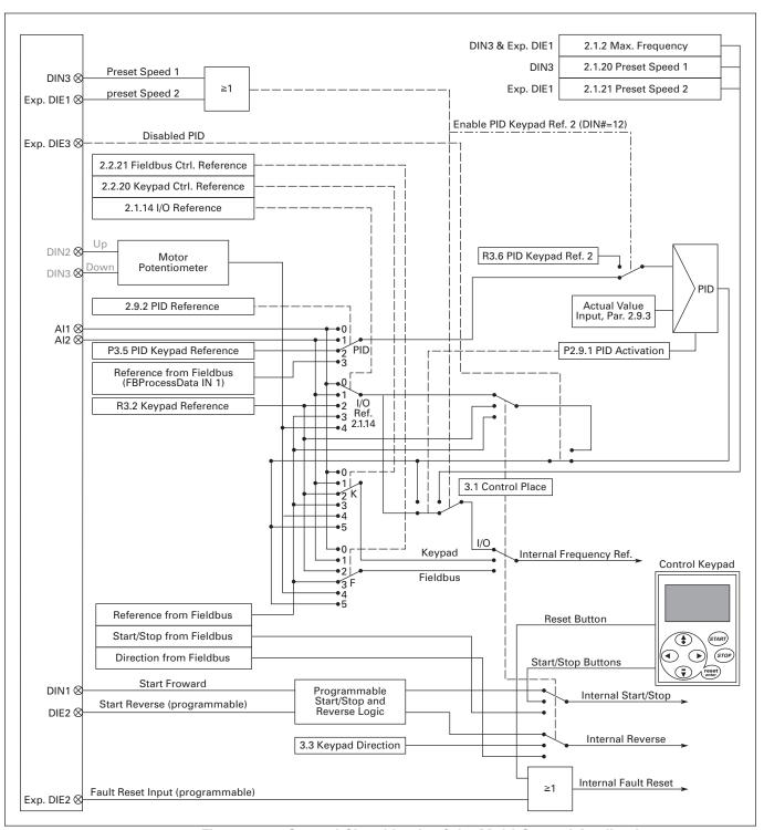
Figure 9-37: Control Signal Logic of the Multi-Control Application
