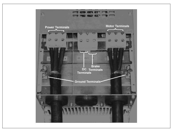
Figure 3-13: Cable Installation in SLX9000, FR7
