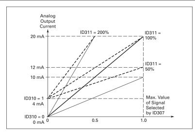
Figure 9-7: Analog Output Scaling
