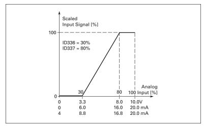
Figure 9-28: Example of Actual Value Signal Scaling
