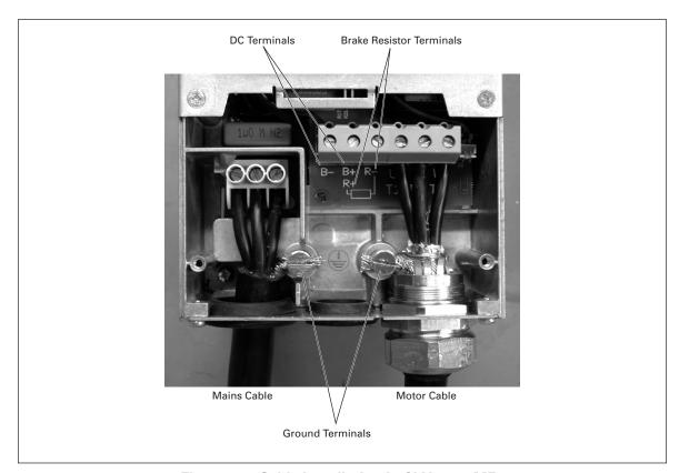
Figure 3-9: Cable Installation in SLX9000, MF5
