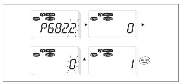
Figure 5-16: MWh Counter Reset
