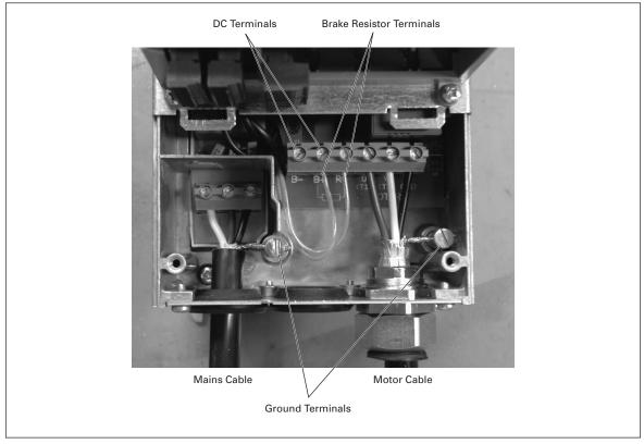
Figure 3-7: Cable Installation in SLX9000, MF4
