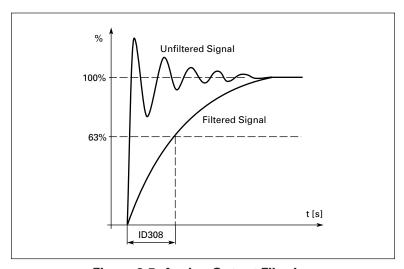
Figure 9-5: Analog Output Filtering
