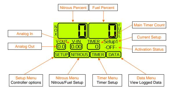
Important Information - Must use Static Suppression Ignition Wires with this Controller. The NMS-1000 Nitrous Controller contains High Frequency Digital Electronics and will NOT function correctly without Suppression Wires!
