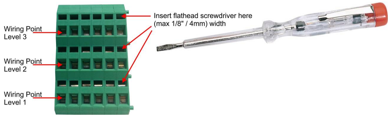
Figure 1.2: Terminal Wiring Details
