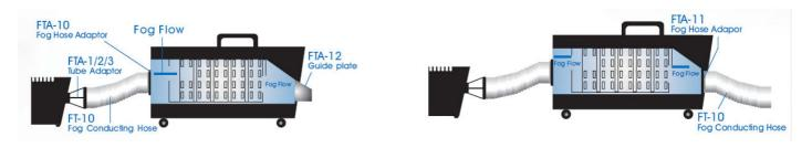
In the first example, a fog conducting hose (FT-10) is attached to a fog machine's output nozzle via an adapter (FTA-1 or FTA-2) and then connected to an adapter (FTA-10) attached to the fog cooler's intake.
