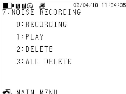
When “ 7. NOISE RECORDING ” is selected from the main menu, the screen shown left appears. You can record, replay, delete, or all-delete the leak noise data collected with the pick-ups. When “ 0. RECORDING ” is selected, the main unit prompts the file number to which the recorded noise data will be saved. After you select the file number, the main unit furthermore prompts you to determine whether the recorded noise data is saved or not. If the current file number is OK, press the Enter key.
