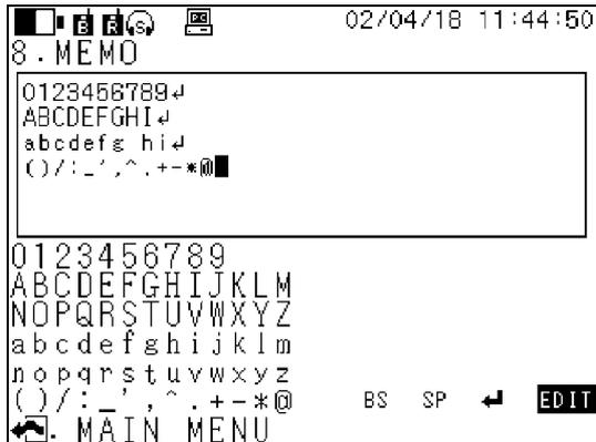
When “8. MEMO” is selected from the main menu, the screen shown left appears. You can enter up to 227 characters showing necessary information, for example, site situation. First, the cursor appears on the alphanumeric table at the bottom.
