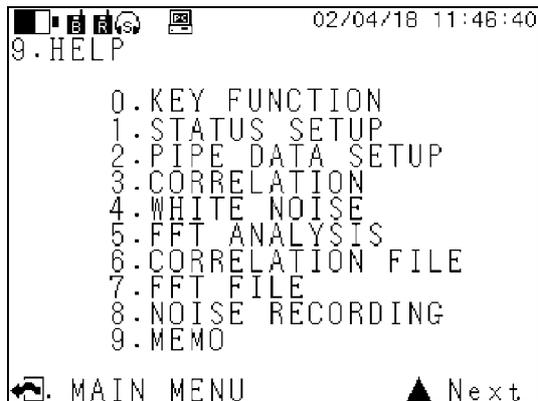
When “9. HELP” is selected from the main menu, the screen shown left appears. This screen contains descriptions about keys and menus. You should use this menu when you are not confident on how to operate the equipment on site. The next paragraph describes the contents.
