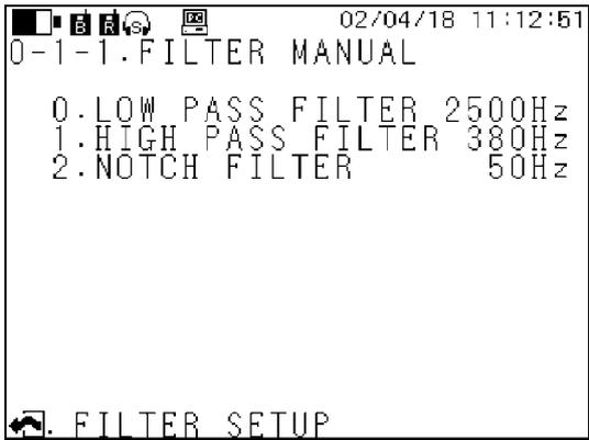
When the manual mode is selected, generally set the filters by referencing the following examples.
