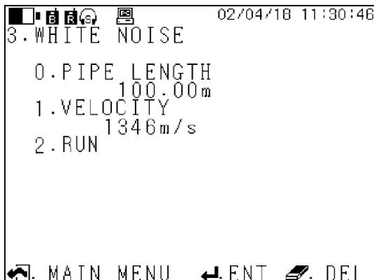
When the pipe data is incomplete, you can measure the pick-up-to-pick-up distance and the sound velocity of the leak noise through this menu to complement the data.
