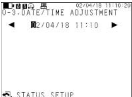
The cursor appears. Move the cursor to the parameter you want to change and enter the value. Then, press the Escape key. The previous screen reappears. This sets the new date and time.
