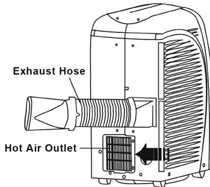
The hot exhaust air can be vented through the wall or out a window. If mounting in the wall, the height of the hole should be 16 to 50 inches (40cm to 130cm).
