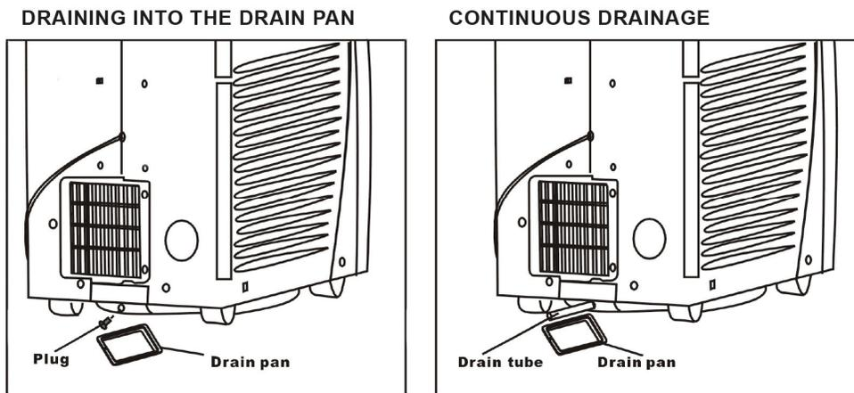
**NOTE:** In heating mode, the drain pipe accessory must be used to empty the water container.
