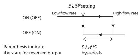
(3) When  $\text{E}03$  is set to  $03$  or  $05$  (within range for instantaneous flow rate)
