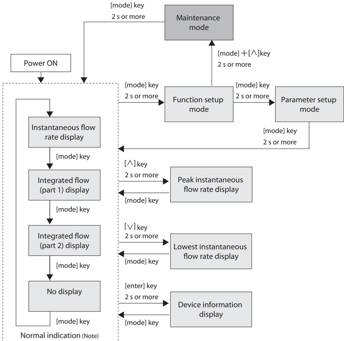
Note Normal indication means display of the instantaneous flow rate, integrated flow last five digits, integrated flow first four digits, or no-display, depending on the setting of function setup  $\text{E}04$ . If an alarm occurs, the alarm code and normal indication alternate every two seconds. For no-display mode, the alarm lights continuously.
