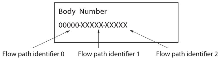
Note Registering the wrong numbers for model number and flow path identifier may result in incorrect display of the flow rate.
