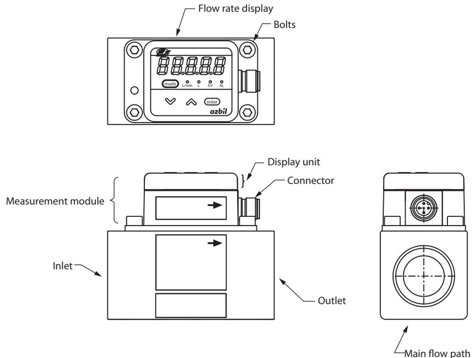
**Flow rate display:** This 7-segment LED indicates instantaneous flow rate or integrated flow amount. For the integrated flow, the first 4 digits and last 5 digits are displayed separately. The 7-segment display also indicates settings in setting mode and alarm codes when an alarm occurs.
