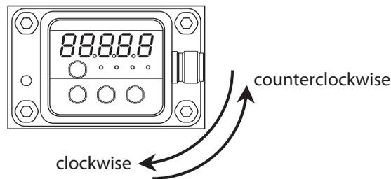
If the display is rotated beyond the range of movement stated above, the internal connector may be disconnected, disabling the display unit.
