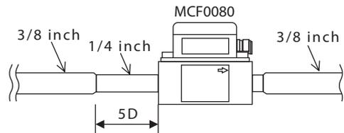
When connecting the MCF to a pipe 1 size larger than the MCF port (for example, the MCF0080 to a 1/2 inch pipe), to determine the straight pipe length, use the section of the table marked "Pipe one size larger in dia. (connected with reducer)."
