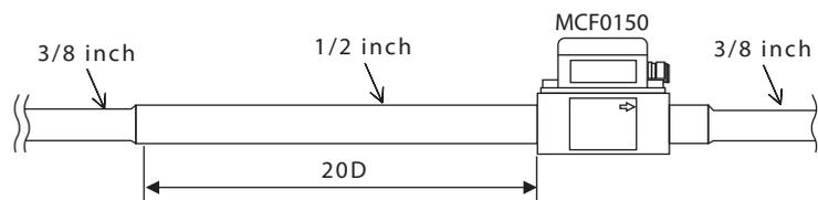
Do not connect a smaller size pipe to the MCF without a straight pipe section. Doing so might cause a reverse flow in the measurement module, even though there is a regular forward flow in the main flow path. Therefore the display might indicate a negative value or an extremely low flow rate compared with the actual rate.
