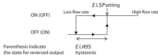
Note If the Event OFF point is less than zero, the output turns off at zero.
