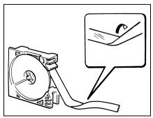
4 An excessively curled film leader results in the Film Supply Reel failing to advance the film smoothly. By studying the illustration on the right, check to see if the curl of your film is up to the specified allowance.
