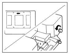
To rotate the image, turn the Prism Rotation Knob.
