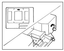
To reverse the film manually, Manual Film Advance Knob and, turn it counterclockwise.
