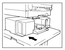
2 Plug the Cable Connector of the Carrier into the Socket in the machine dedicated to this Carrier.
