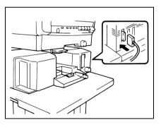
3 Install the Lens Unit all the way into Position.
