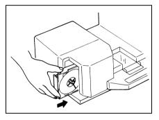
2 When the Cartridge is properly inserted into position, the film leader is automatically unwound and taken up by the Take-Up Reel.
