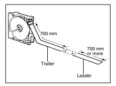
2 Keep the edge of the leader cut straight, especially when the edge is folded, to ensure that the film is unwound smoothly.
