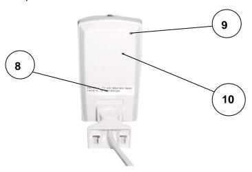
**Remark:** No. 9 and No. 10 are used for the control of PIR sensitivity and duration time respectively. Please adjust these parameters in the clockwise/counterclockwise direction to increase/decrease the setting values.
