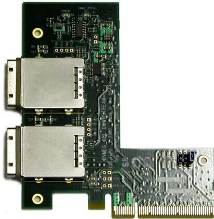
The board fits into any 8x or 16x PCI Express slot. Make sure the computer is powered off when you install the board into it. There are two x4 cable connectors on the board. You should use only the bottom one with the DNV7F2A because the DNV7F2A PCI Express interfaces only support 1x or 4x PCI Express links. The top connector on the PCI Express cable adapter card is for use with 8x links.
