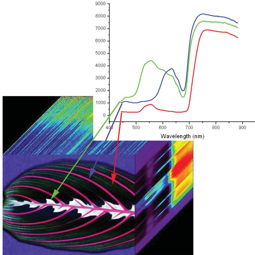
Hyperspectral imaging has a long heritage as a remote sensing tool, operating from satellites and airplanes. In this capacity, it has proven itself as a useful tool for scene discrimination; the Pika series imaging spectrometers provide this powerful capability in a cost-effective, compact package.
