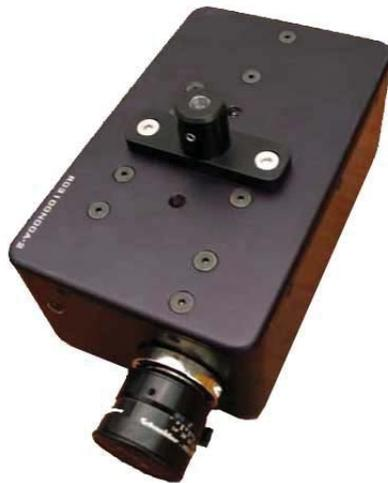
Second, attach the Pika imaging spectrometer to the Rotation Stage and tighten the set screw in the Rotation Stage mounting bracket.
