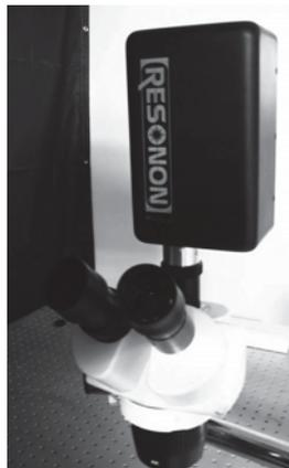
Adjust the focus of the microscope while viewing the focusing object through the microscope's eyepieces. Then, adjust the focus on the camera port of your microscope until the instrument is focused simultaneously.
