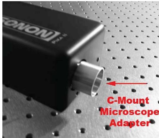
Second, mount the Pika II on the camera port of your microscope and lock down the set screw in the C-Mount Microscope adapter.
