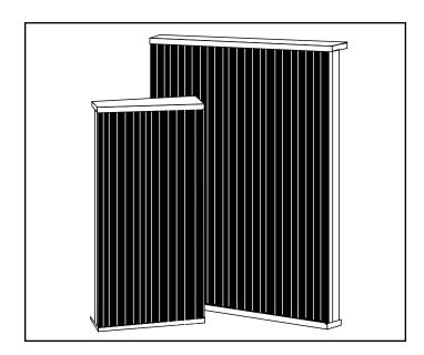
The RAYMAX® 1120 is a lightweight, yet sturdy and durable radiant heater panel. The emitter sheath is stainless steel with a black coating that makes it a highly efficient radiating surface. In addition, the heater's low mass allows rapid start-up and fast response to controls.
