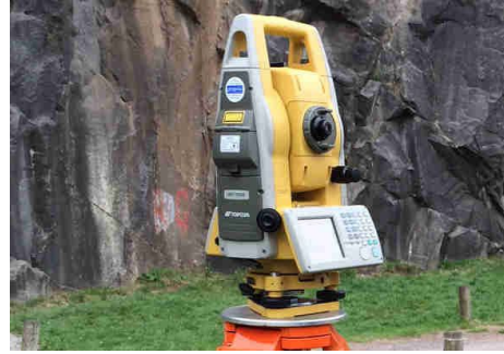
Figure 6: The equipment used to survey in Ground Control Points.
