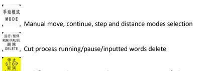
High/low speed parameter adjust, Cut process stop/selections, inputting and operating cancel
