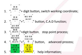
There are some compound buttons for special applications. The operating mode is: press the first button and hold then press the second button, release the two buttons at same time.
