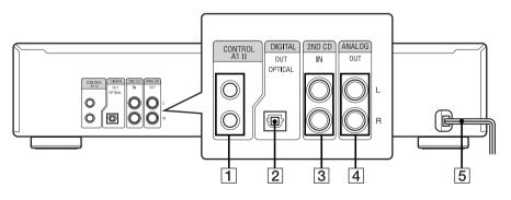
2ND CD IN jacks 3 (8) ANALOG OUT L/R jacks 4 (6) CONTROL A1II jacks 1 (6, 20) DIGITAL OUT OPTICAL jack 2 (7) Mains lead 5 (6)
