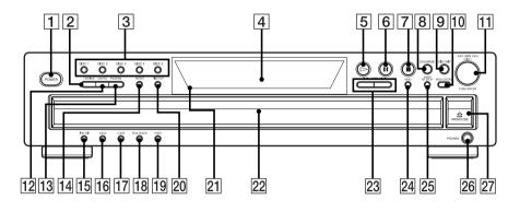
CHECK 16 (13) CLEAR 17 (13, 14, 16, 17) CONTINUE 2 (9, 13, 15, 18) DISC 1-5 3 (9, 10, 13) Disc compartment 22 (9) DISC SKIP 9 (9, 12, 13) Display 4 (11) EX-CHANGE 8 (12, 15) FADER 19 (14, 20) MEGA CONTROL 10 (18, 19) MENU 24 (8, 16, 17) PEAK SEARCH 18 (15) PHONES jack 26 (10) POWER 1 (7, 9, 16) PROGRAM 13 (9, 13, 18) Remote sensor 21 (6) REPEAT 14 (10, 18) SHUFFLE 12 (9, 10, 18) TIME EDIT 15 (14) TIME/TEXT 20 (11) X-FADE/NO DELAY 25 (19, 20)
