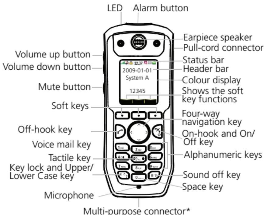
\*) Used for battery charging, configuration and connection of headset connector.
