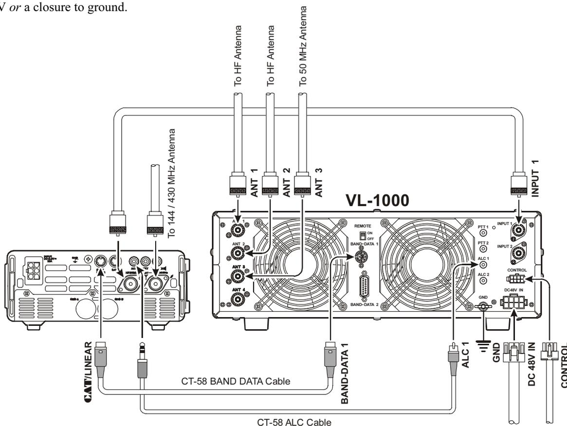
\*The “CT-58” consists of two separate cables: the BAND DATA cable (Part # T9101500) and the ALC Cable (T9101501).
