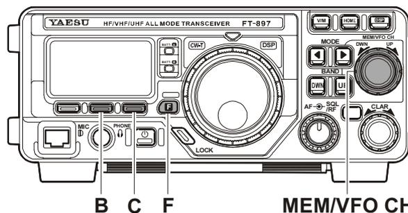
1. Press the **[F]** key momentarily, then rotate the **MEM/VFO CH** knob, as needed, until Multi Function Row “I” [NB, AGC, AUTO] appears on the display.
