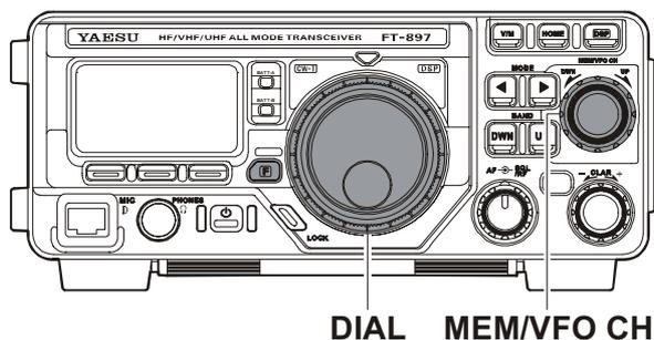
The synthesizer steps for the **MEM/VFO CH** knob may be adjusted independently by mode. Use Menu Mode No-006 [AM STEP] for AM, No-052 [FM STEP] for FM, and No-082 [SSB STEP] for SSB/CW/Digital. See pages 56, 59, and 62 for details.
