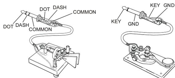
**Note:** Even when using a straight key, you must use a three-conductor (“stereo”) plug. If a two-conductor plug is used, the key line will be constantly shorted to ground.
