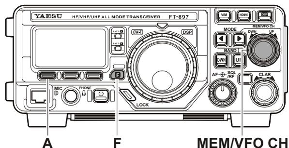
Now press the [**A**](A/B) key to toggle between the “A” and “B” VFOs. There are two such VFOs provided on each Amateur band, so you may set VFO-A to the CW sub-band, and VFO-B to the SSB sub-band, if you like. The operating mode will be preserved, along with the frequency information, on each VFO.
