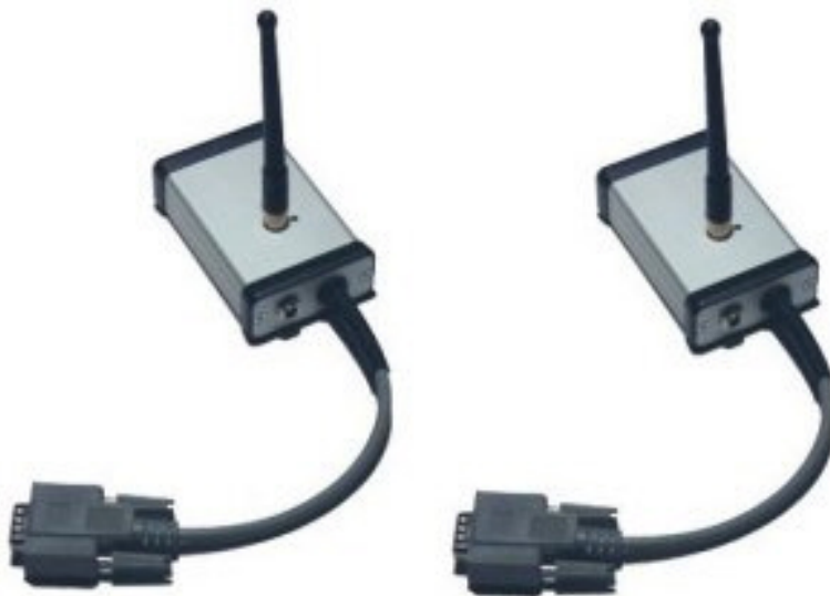
Figure 2.3.2 BlueWave Industrial Wireless Cable [Ref 4]
