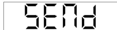
This display shows that Selcall is being sent - ie. in transmit mode.
