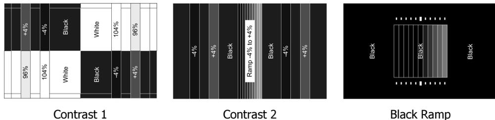
For white level the 96% and 104% vertical bars should be differentiable from the 100% background, and the 104% bar should not be "crushed" which may show as a color change versus the 100% background and 96% bar. Use the Radiance "Contrast 1" and "White Ramp" patterns.
