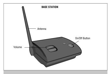
**On/Off:** To turn the Base Station on and off, hold down the power button until you hear the on/off tone.
