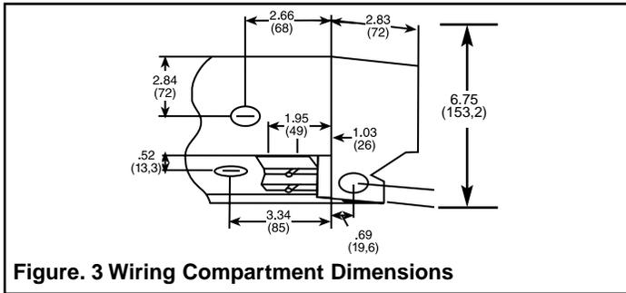
Figure 3 Wiring Compartment Dimensions
