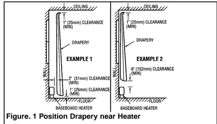
Figure. 1 Position Drapery near Heater
