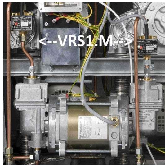
Figure 26 – Vapor recovery with vapor flow sensor VRS1.M
