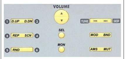
**D.UP** ~ **D.DN**: Press to move to the next or previous disc. **REP** ~ **SCN**: Press REP to repeat the current disc. Press SCN to play the first ten seconds of each track on the selected disc. **RND**: Press to randomly play tracks on the selected disc. **Volume:** UP/Down on volume button is used to control the sound level of the CD Player and Radio. This button also is used to control the level of Bass, Treble and speaker balance in each respective mode.
