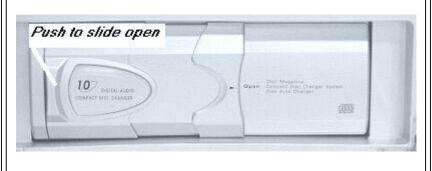
To load the magazine into the CD player, slide the door to the right as shown in the photos. Check to make sure that you have the magazine positioned so that the top side is up and that it is pointed in the right direction for installation. You should be able to see the writing and disc numbers on the front after it is inserted.
