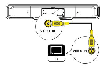
1 Connect a composite video cable (supplied) from the VIDEO OUT socket on this unit to the video input socket on your TV.
