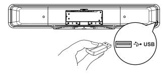
1 Connect the USB device to ↔ (USB) socket on this unit.
