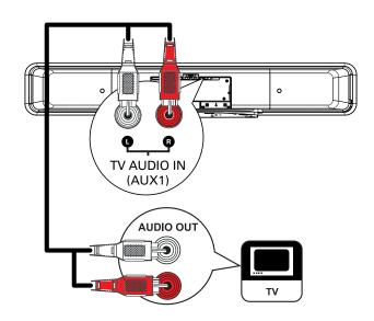
1 Connect an audio cable (not supplied) from the TV AUDIO IN (AUX1) sockets on this unit to the AUDIO OUT sockets on your TV.
