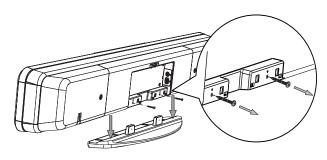
**3** Attach the supplied knobs to the rear of this unit.
