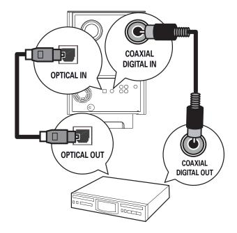
1 Connect a coaxial cable (not supplied) from the **DIGITAL IN-COAXIAL** socket on the subwoofer to the COAXIAL/ DIGITAL OUT socket on the device.
