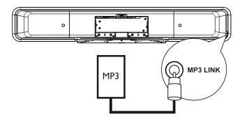
1 Connect a 3.5mm stereo audio cable (supplied) from the **MP3 LINK** socket on this unit to the phone socket on your portable media player (such as MP3 player).
