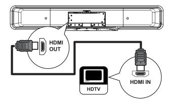
1 Connect a HDMI cable (supplied) from the HDMI OUT on this unit to the HDMI IN socket on your TV.
