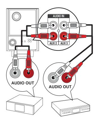
1 Connect an audio cable (not supplied) from the AUDIO IN-AUX2 or AUX3 sockets on the subwoofer to the AUDIO OUT sockets on the device.
