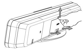
2 Connect the cables to the corresponding sockets and direct the cables to the CABLE OUT point.
