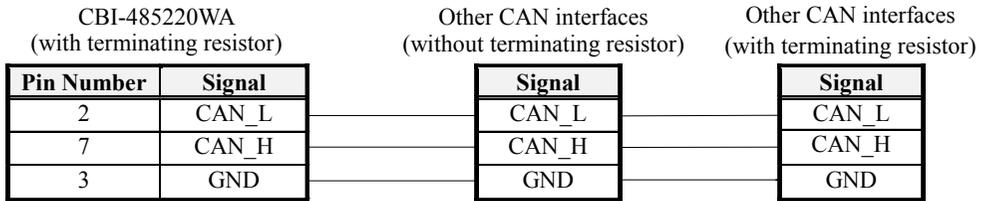
Note: To avoid an error, connect a CAN Interface with terminating resistor to the both ends of the network.
