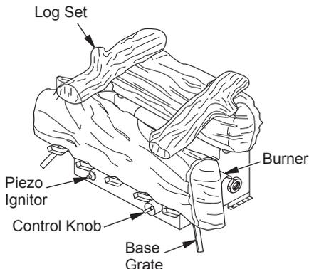
**Figure 1 - Vent-Free Gas Log Heater**
