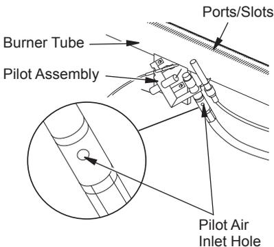
Figure 37 - Pilot Inlet Air Hole
