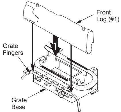
**Figure 19 - Installing Front Log #1
