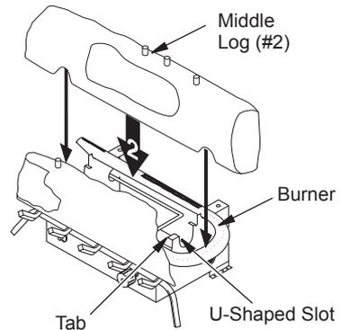
**Figure 20 - Installing Middle Log #2
