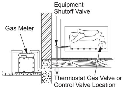
**Figure 18 - Checking Gas Joints (Natural Gas Models)**
