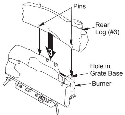
**Figure 21 - Installing Rear Log #3
