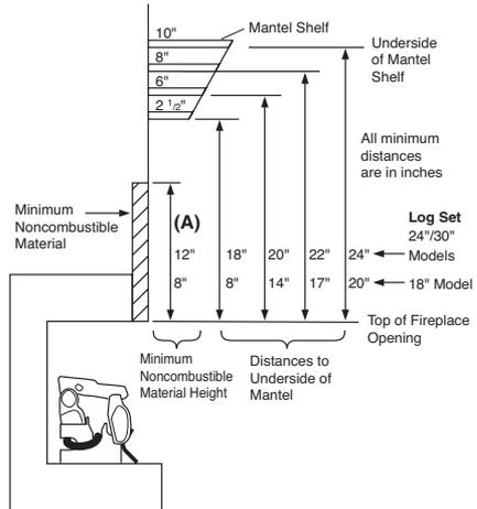
**Figure 6 - Minimum Mantel Clearances Without Using Hood**
