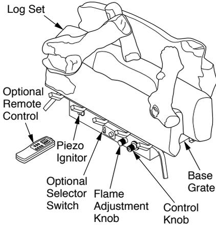
**Figure 1 - Vent-Free Gas Log Heater
