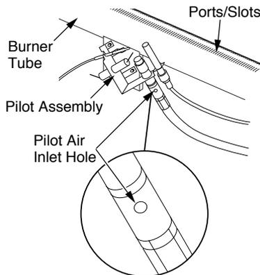
**Figure 40 - Pilot Inlet Air Hole**
