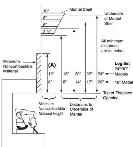
**Figure 6 - Minimum Mantel Clearances Without Using Hood**
