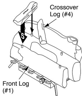
**Figure 29 - Installing Crossover Log (#5)**
