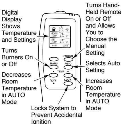
**Figure 36 - Thermostat Hand-Held Remote Control Unit (GHRCTB)**
