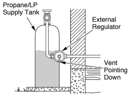
**Figure 13 - External Regulator With Vent Pointing Down**
