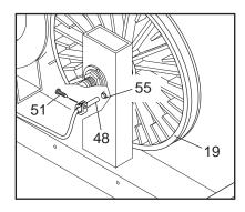
for clarity). Slide the Reed Switch slightly toward or away from the Magnet. Make sure that the Magnet will not hit the Reed Switch. Retighten the Screw. Turn the Pulley (19) for a moment. Repeat until the console displays correct feedback. When the Reed Switch is correctly adjusted, re-attach the left side shield.
