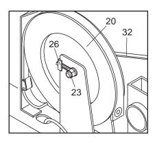
counterclockwise. Make sure that the Flywheel is straight and retighten the M8 Flange Nuts (23). When the Drive Belt is properly adjusted, re-attach the side shields.
