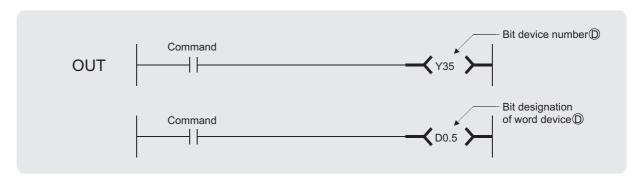
① : Number of the device to be turned ON and OFF (bits)
