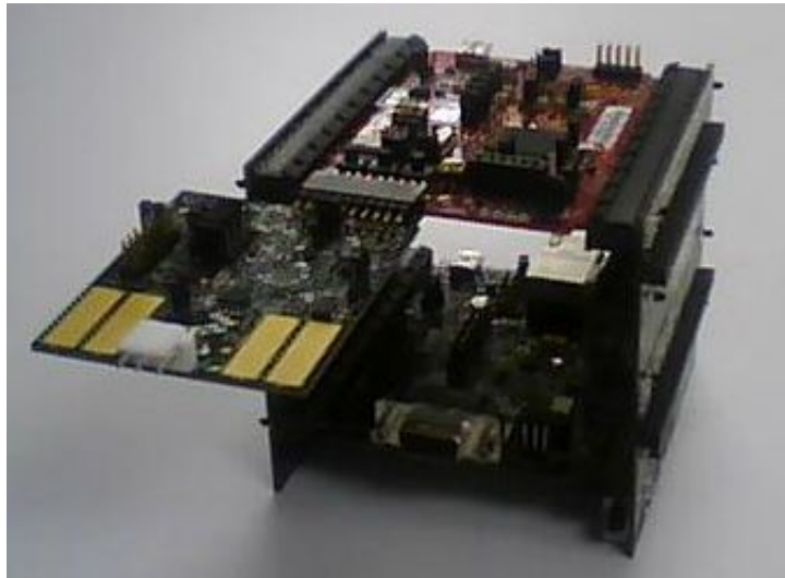
Figure 27. Tower system assembled for the MED-EKG demo
