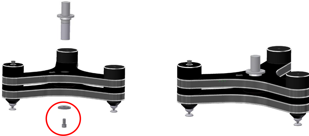
Pic. 6: Set – up of the drive bearing
