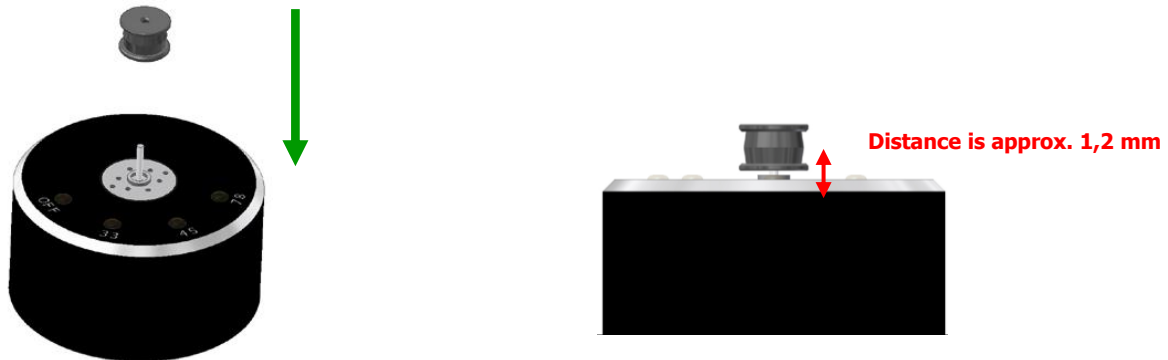
Pic. 7: Set – up of the Master Innovation pulley
