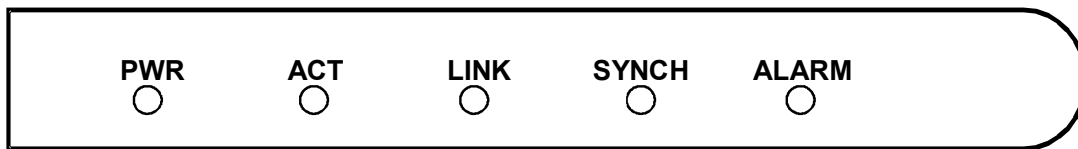
Fig. 19 FG-PAM-SAN-4Eth-R,V1 front panels
