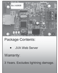
WEB SERVER MONITORS AND CONTROLS JVA ENERGIZERS VIA THE INTERNET
