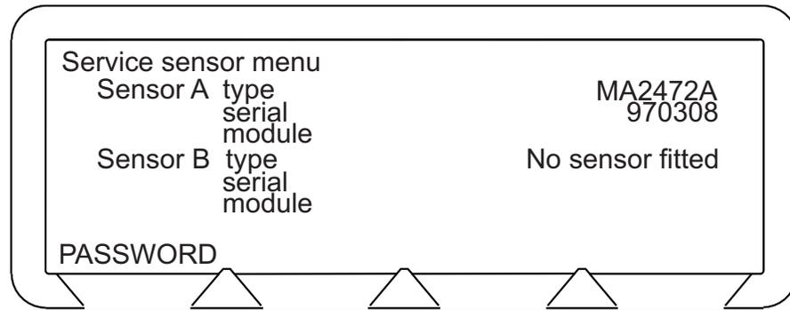
The example display above shows an ML2438A (dual channel) meter with an MA2472A power sensor connected to input A, and no sensor connected to input B. A single channel meter (ML2437A) will only show the Sensor A information.
