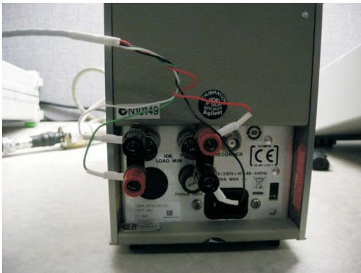
Connection shown to the rear of the 432A power meter:
