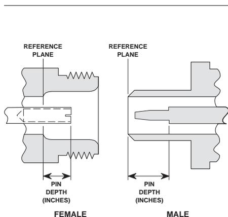
The center pin of a precision RF component connector has a precision tolerance measured in mils (1/1000 inch). The mating connectors of various RF components may not be precision types. Consequently, the center pins of these devices may not have the proper depth. The pin depth of DUT connectors should be measured to assure compatibility before attempting to mate them with Power Meter or sensor connectors. An ANRITSU Pin Depth Gauge (Figure A-), or equivalent, can be used for this purpose.
