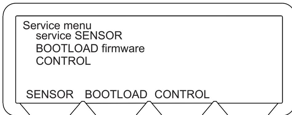
The SENSOR service mode is detailed in the following section of this chapter. BOOTLOAD mode is covered in Chapter 5, and the CONTROL mode is used in manufacturing and not required by service personnel.
