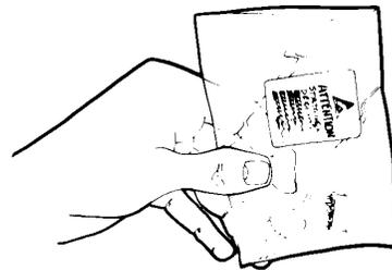
9. Transport and store PCBs and static sensitive devices in static-shielded containers.
