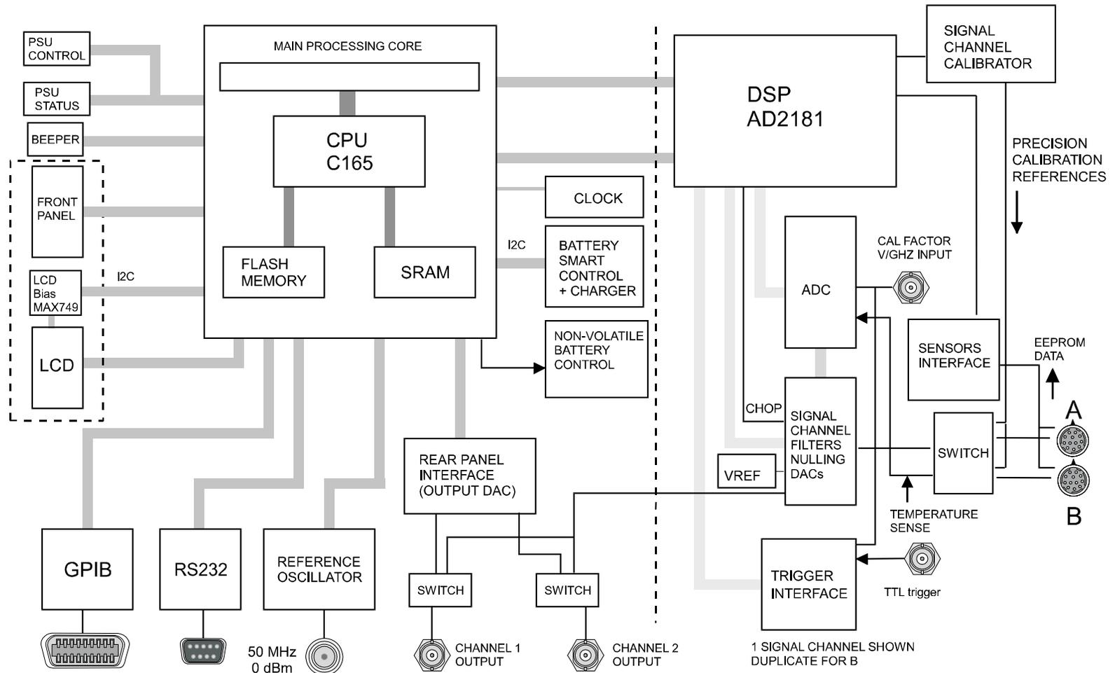
Figure 4-1. ML2430A Series Power Meter Functional Block Diagram
