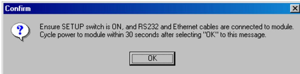
14. Click *OK*, **Power down** module, wait approximately 1 second, and power up module. This entire step must be accomplished within 30 seconds of completing the previous step.
