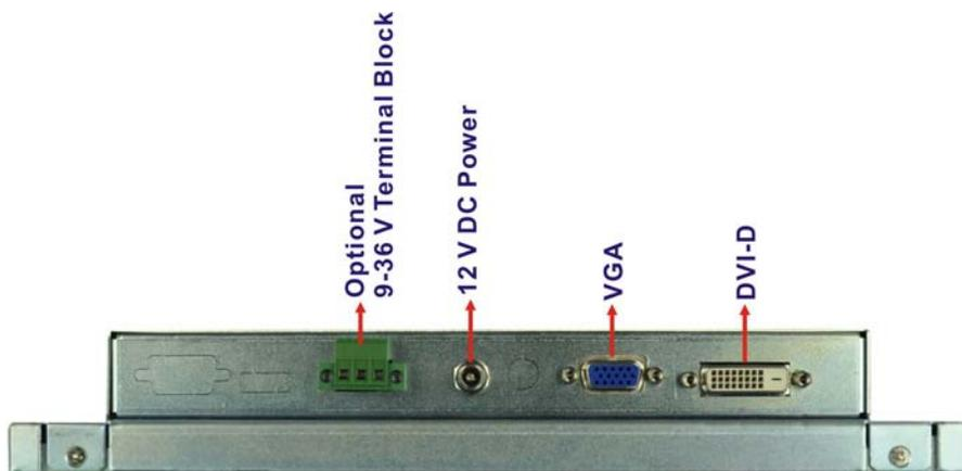
Figure 1-4: Typical LCD-KIT Connectors
