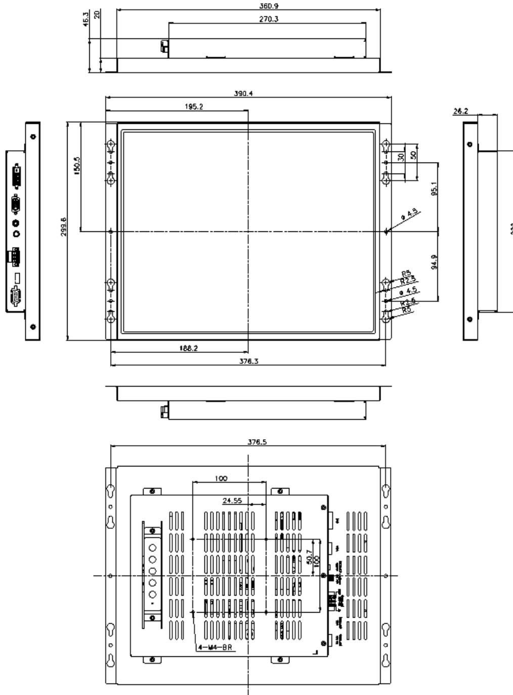
Figure 2-3: LCD-KIT170G Physical Dimensions (millimeters)
