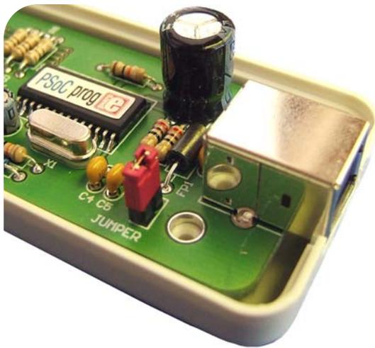
This picture shows the position of jumper when the target board and *PSoCprog* programmer are powered trough USB connector.
