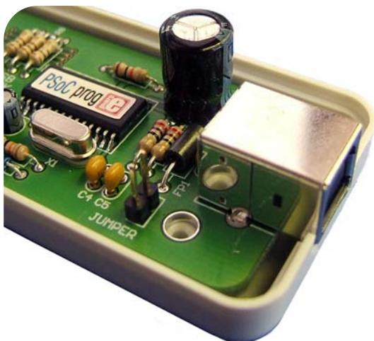
This picture shows the position of jumper when *PSoCprog* programmer is powered by the target board.
