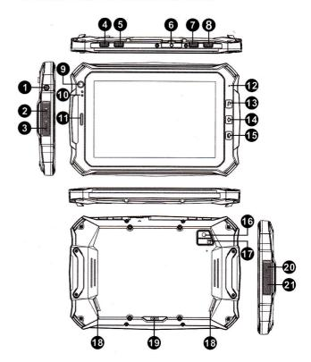
1: Reset: Poke the reset hole to reset the system.
