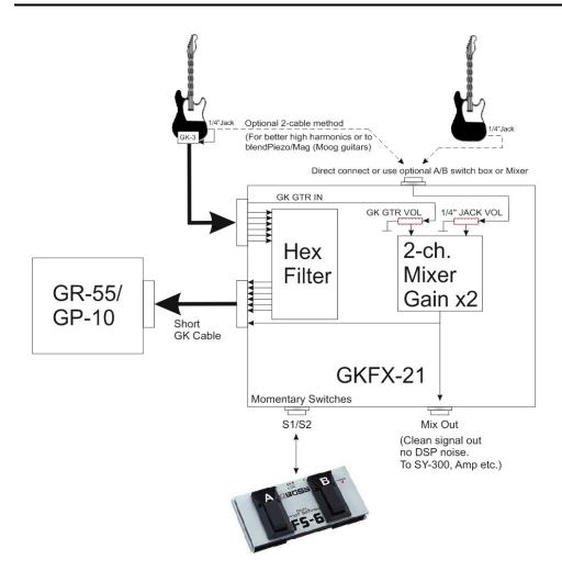
The GKFX-21 is to be connected between a 13-pin guitar and a synth unit. The synth unit provides power to the GKFX-21.
