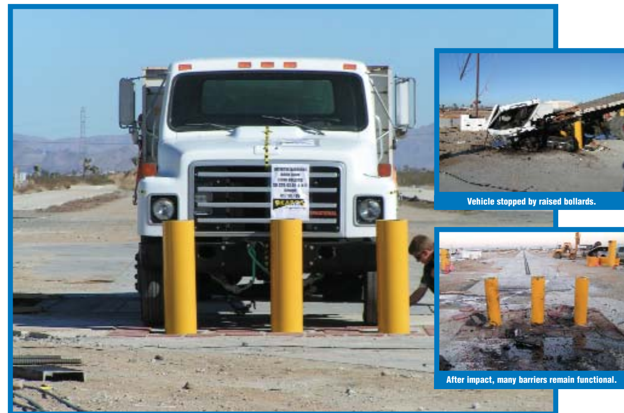
Bollards, in fully guarded position, consist of a series of large retractable steel obstacles.
