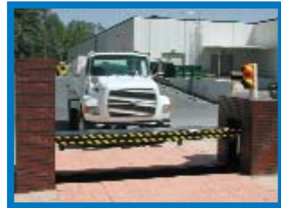
Necessary with each barrier type, the horizontal beams render vehicles totally inoperable.
