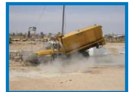
Anti-terrorist barriers are capable of stopping vehicles running 50 mph.
