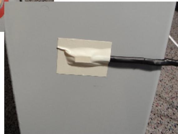
**FIGURE 16.10.7.** Temperature switches showing connections to TOP and SIDE. Up to 24 locations may be used.
