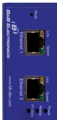
Figure 4. Ethernet Connector
