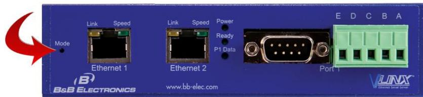
Figure 3. Front View of the Serial Server
