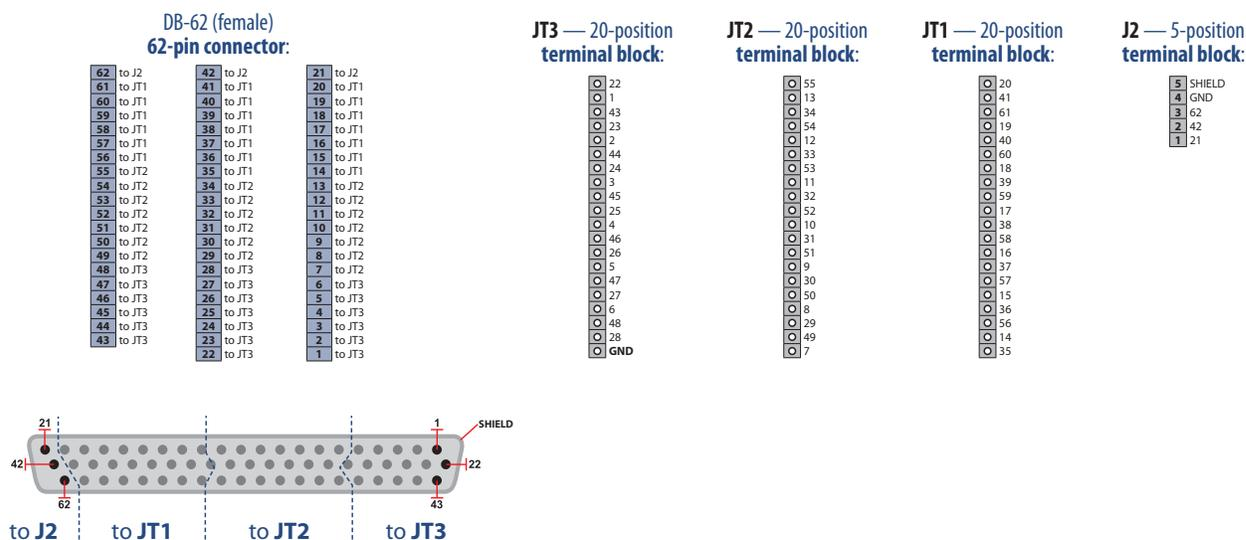
**Figure 1-9. Layout of DNA-STP-62 Screw Terminal Panel**
