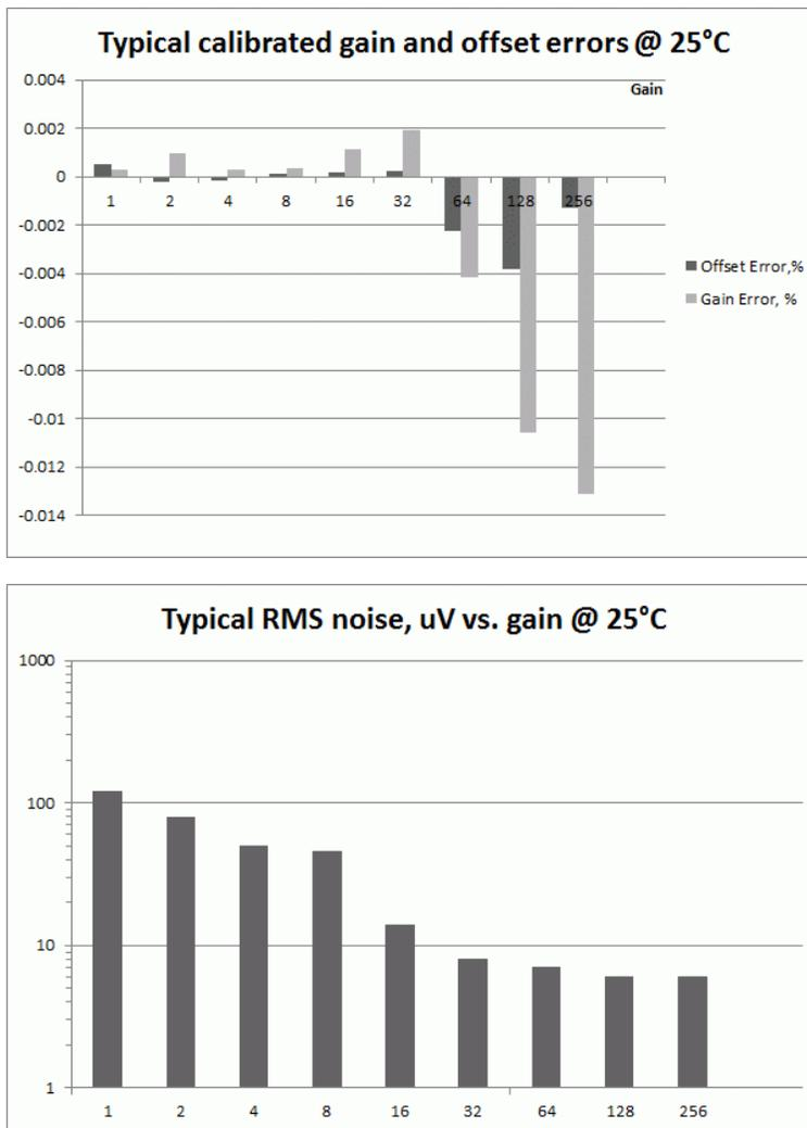
**Figure 1-1. Offset error and RMS noise vs. gain**
