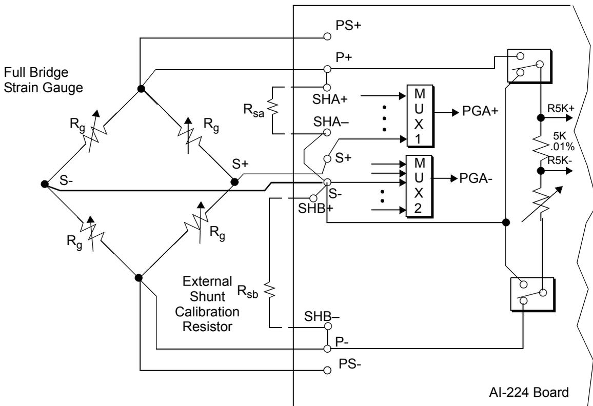
**Figure 1-6. Full Bridge Strain Gauge Circuit.**
