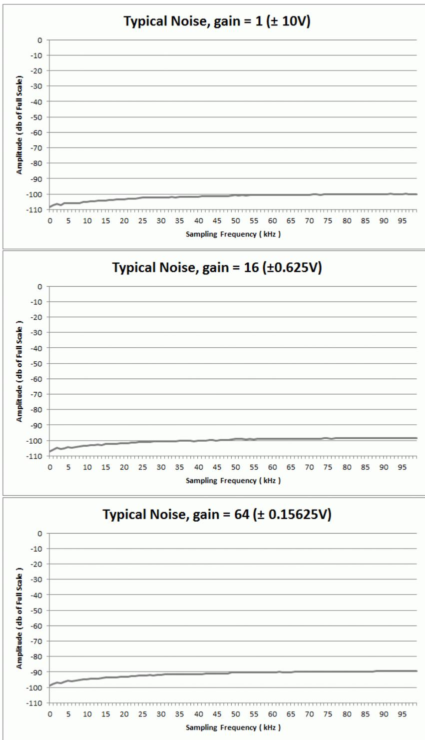
**Figure 1-2. Noise amplitude at various sampling rates**
