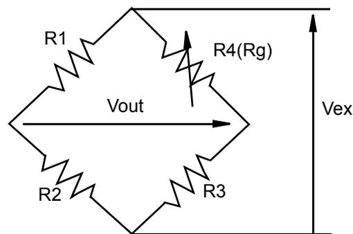
**Figure B-1. Strain Gauge Bridge**
