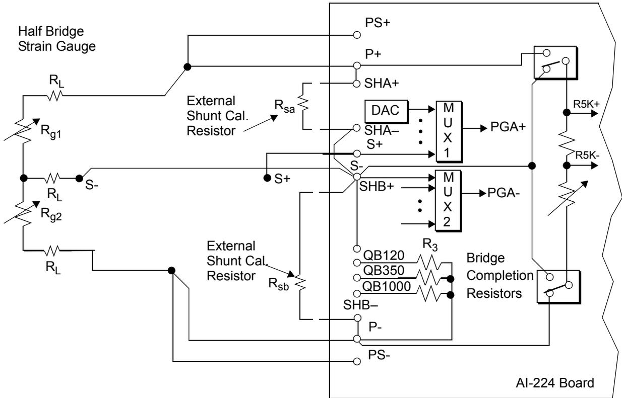
**Figure 1-7. Half Bridge Strain Gauge Circuit.**
