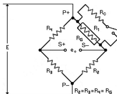
**Figure 1-10. Shunt Calibration**
