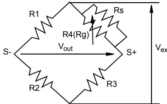
**Figure B-2. Strain Gauge with Shunt Resistance  $R_s$  Added**
