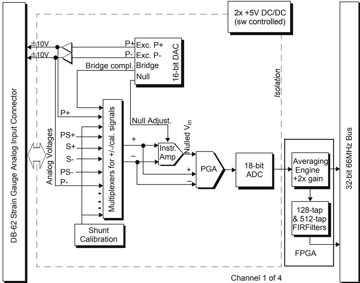
**Figure 1-3. Block Diagram of the AI-224 Layer**
