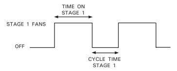
Stage 1 fans run during time on. The Stage 1 Pilot Light turns on. During time off, the Stage 1 fans do not run. The Stage 1 Pilot Light turns off.
