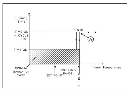
This option is activated by setting internal switch # 8 to OFF. When the temperature is less than the set point + timer temp. range, Stage 1 fans run according to the minimum cycle (see above). When the room temperature reaches point A, stage 1 fans run continuously with no transition.
