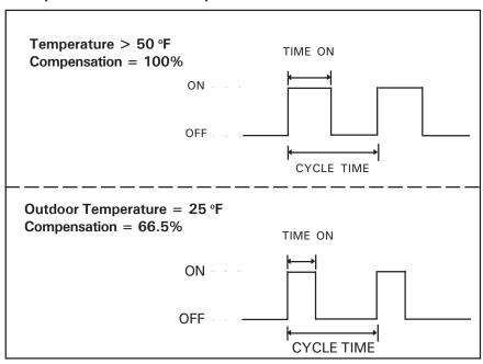
In the first example given on the following page, compensation is not needed when the outside temperature is greater than 50 °F. The fans operate according to the full running time defined by the parameter settings. In the second example, the running time is decreased to 66.5% of full running time to compensate for the colder outdoor temperature. Cycle time remains unchanged.
