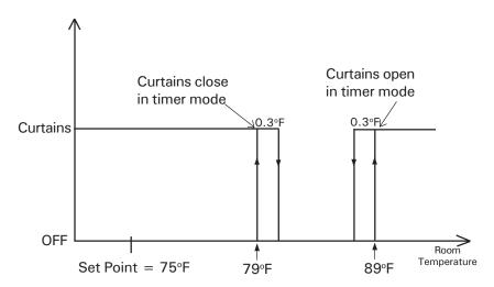
In the example above, when the temperature rises to 89°F, the sidewall and endwall curtains begin to open and continue to do so until fully open if the temperature remains above this point. If the temperature falls to 88.7°F, the curtains stop opening.
