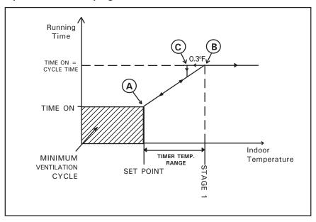
This option is activated by setting internal switch # 8 to ON. At room temperatures at or below the set point, the controller operates the Stage 1 fans according to the minimum ventilation cycle.
