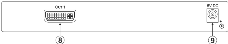
Figure 2: VM-200HDCP 1:2 DVI Distributor Rear Panel
