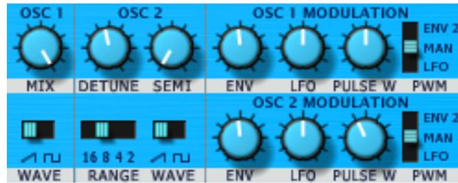
The controls that determine the pitch and waveform of the oscillators and how they react to modulation are in this area.
