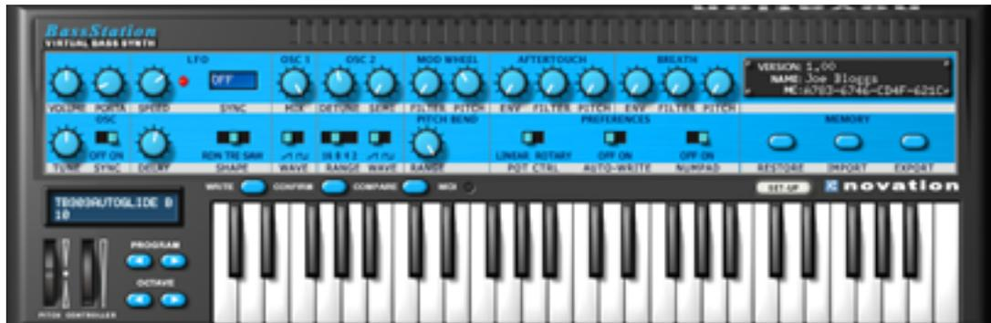
Just over half the panel changes to show not only some lesser used sound creation parameters but some options and preferences that affect overall operation of the BassStation. It's in the SETUP pages as well where you can restore the factory presets and import / export sounds from / to either a keyboard BassStation or a BassStation Rack module.
