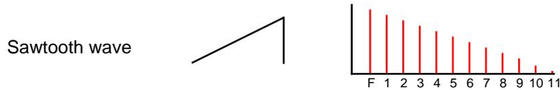
The sawtooth wave is probably the brightest sounding waveform of all and contains a wide range of odd and even numbered harmonics in equal proportion. It is good for a wide range of sounds including strings, brass and more.
