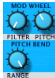
The FILTER control determines how much the mod wheel will open and close the filter's cutoff frequency.
